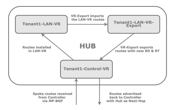
In a spoke-to-spoke via hub topology, the branches communicate only through the hub. The IP prefixes of remote branches always have the hub as the next hop.
