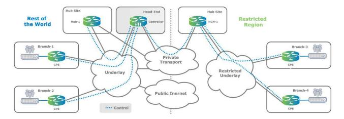
You can apply the SD-WAN network topology shown in the following figure to restricted regions. Branches in this region create an SD-WAN island in the form of a restricted underlay that has no connectivity with the rest of the world. An approved transport must be provided by a government-approved service provider to allow IPsec traffic, which can be a
