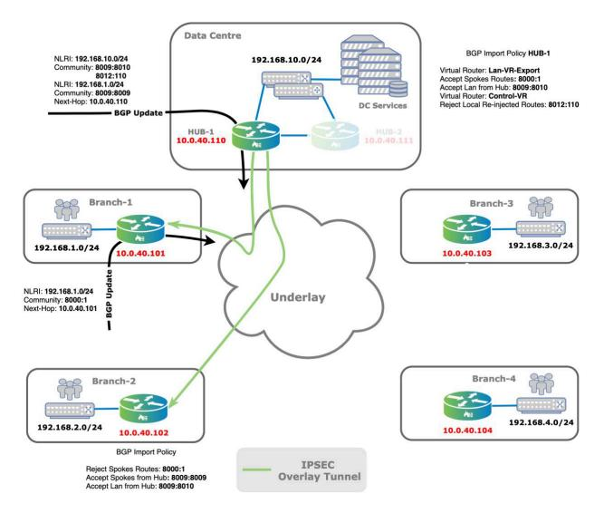
You can use the spoke-to-spoke through a hub topology when communication between branches is not required, for example, when security and other services are centralized at the hub site or when the cost of ownership of WAN links dictates it.
