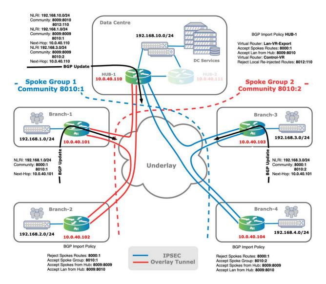
For a spoke-to-spoke–direct topology, you use spoke groups. Branches within the same spoke group can communicate directly with each other, and they use hubs to reach branches in different spoke groups. In the topology shown above, Branch-1 and Branch-2 communicate with each other directly, but to reach Branch-3 the next hop is Hub-1. The hubs are connected using a full-mesh topology.
